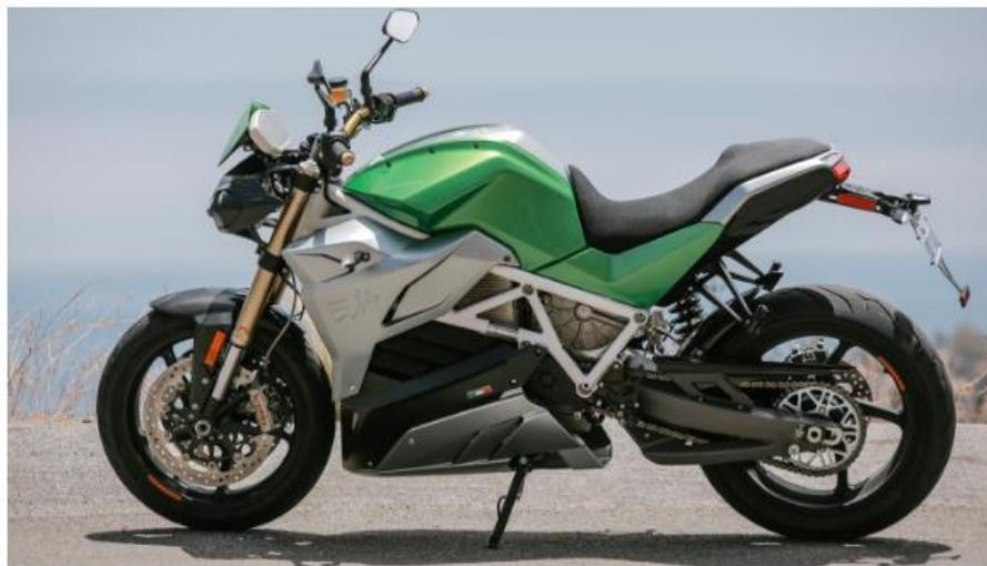
What separates the Energica from other electric motorcycles is its integrated fast-charge system. The under-seat outlet is fully compatible with commercial recharging stations, or the bike can be charged at home with a traditional wall outlet. The advantage of the fast-charge system is the greatly reduced time required to recharge the battery (versus slower times ... often the bane of electric vehicles) with the 4 DC system restoring up to 85 percent of battery power in just 30 minutes.
