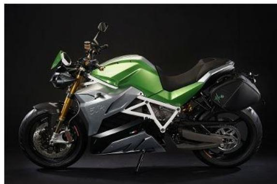
Energica Eva, the second model of the Italian manufacturer unveiled in its final version at EICMA 2015, is equipped with a permanent magnet AC (PMAC) oil cooled motor that produces **70kW** (95 hp c.ca) of instantaneous power and a torque of **170 Nm**.
